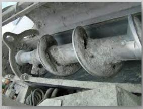
Concrete Screw Feeder
