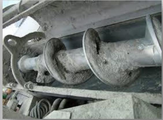
**Concrete Screw Feeder
