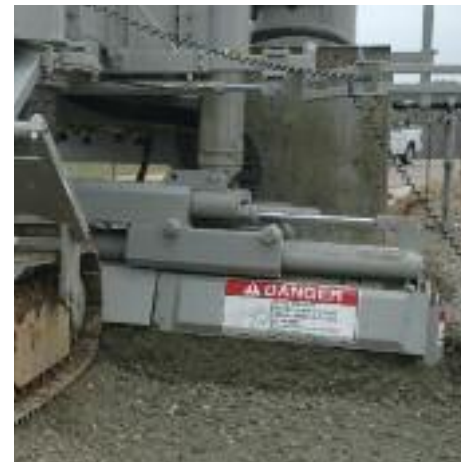
Heavy duty trimmer with extension.
