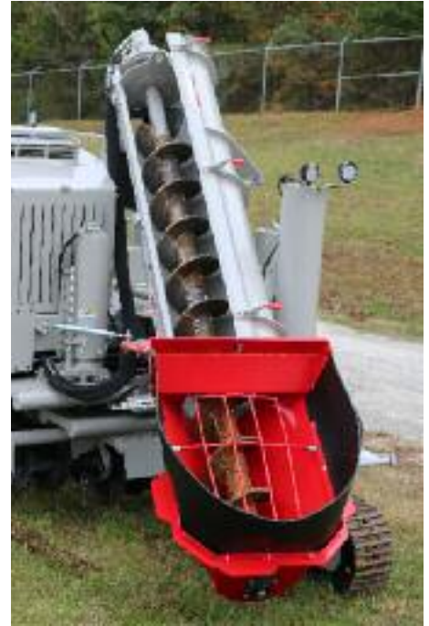
Auger Conveyor; lid opens for cleaning.
