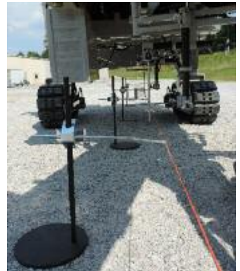
Parapet sensor mounting.
