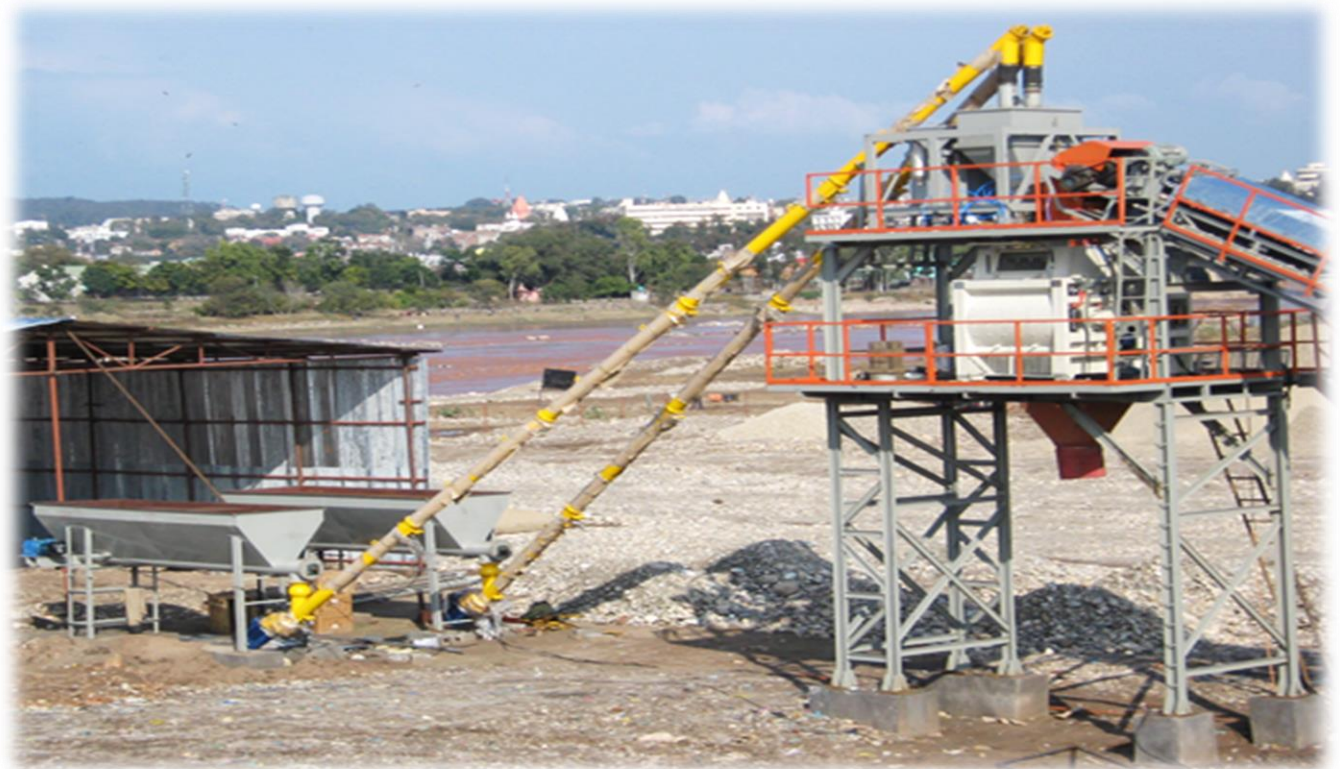
Horizontal Trough Silo to load cement manually into Vertical Silo through Bucket Elevator Or directly discharge cement into the weighing hopper Eliminating need for Vertical Silo.
