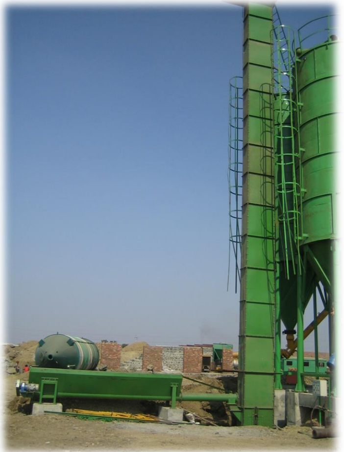
Horizontal Trough Silo to load cement manually into Vertical Silo through Bucket Elevator Or directly discharge cement into the weighing hopper Eliminating need for Vertical Silo.
