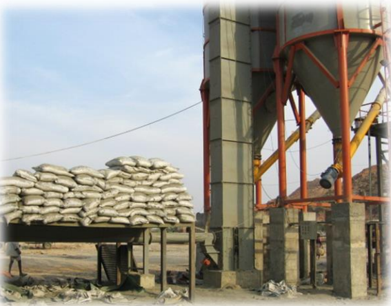
Cement Root Blower Pump with Hopper for manual cement feeding into Vertical Silo or to blow cement from Bulklers into Vertical Silo.
