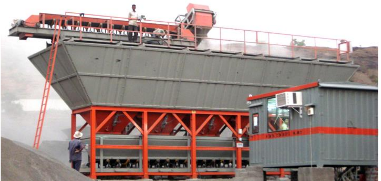
Shuttle Conveyor on top of the Bins
