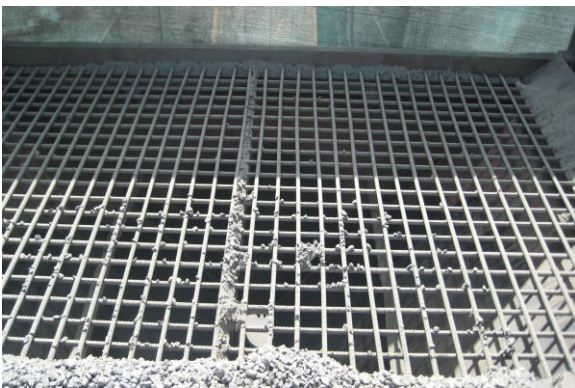
Horizontal Trough Silo to load cement manually into Vertical Silo through Bucket Elevator Or directly discharge cement into the weighing hopper Eliminating need for Vertical Silo.
