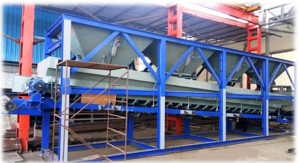
IN-LINE-BINS can be placed on Compacted PCC base. Eliminates costly RCC Column construction and time.
