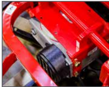
Our super heavy-duty gearboxes have a 20:1 gear box ratio that provides superior rotor speeds.
