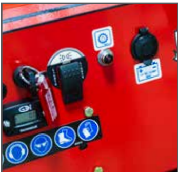
Easy-to-access switches and 12 volt charging plug for phones or electronic devices.
