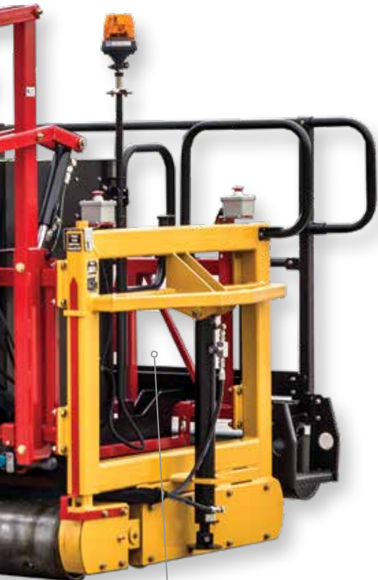
Operator console positioned inside of main frame
