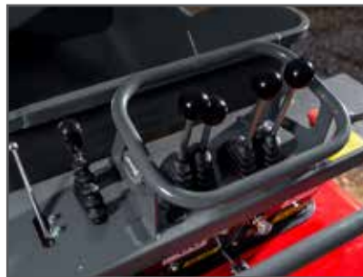
Two servo levers control the direction of the machine, and they automatically reset to stop in case of emergency.
