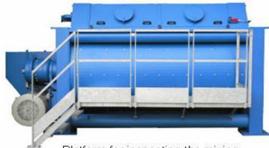
Platform for inspecting the mixing Inside the mixer.
