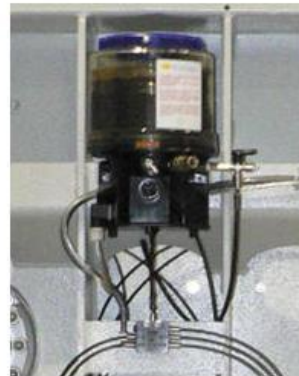
Automatic greasing system
