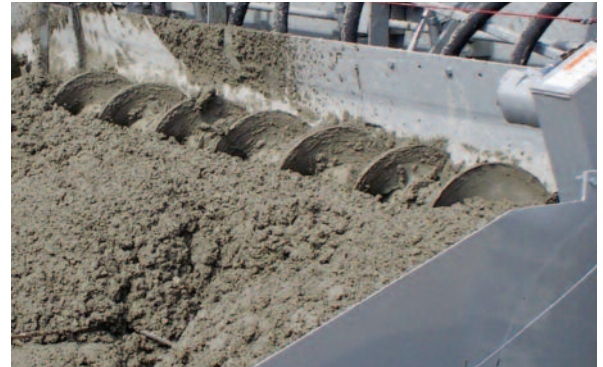
The spread auger and strike-off plate.
