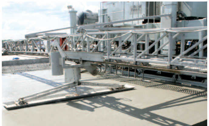
Optional final finisher features an oscillation mechanical float.
