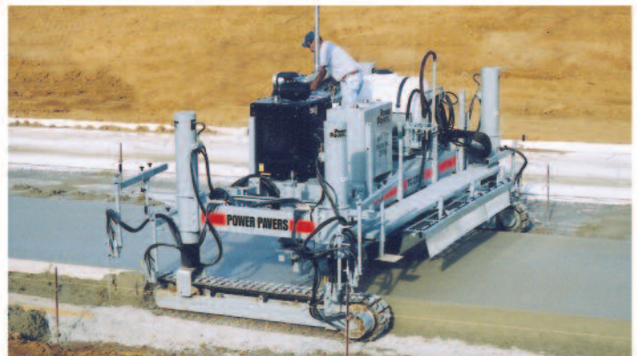
▲ Power Pavers TC-2700 Texture/Curing Machine
