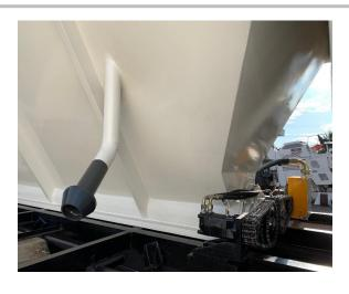
Cement can be pumped from a Bulker directly into the Tank provided with Dust Filter system
