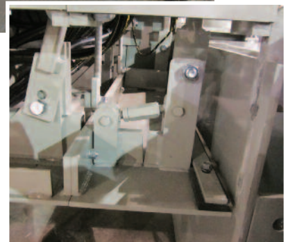
Everything works together to create pavement with a smooth flat finish with a sharp edge (top). Edge overbuild feature compensates for edge slump (bottom).
