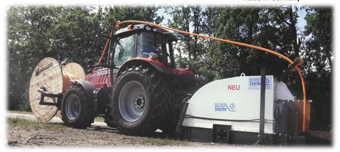
More economical and powerful than a self-propelled cutter. Direct drive via PTO shaft, enormous torque.
